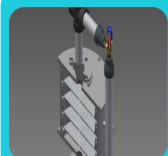
FerryBox flow-through filtering system
